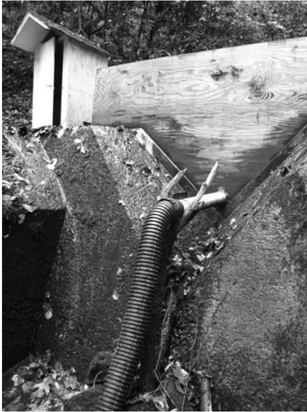
Figure 1. Diversion method used to reduce stream base flow by 50% on average in the experimental drought transects. Baseflow was decreased from 0.24 to 0.10\text{--}0.16\text{ L s}^{-1}\text{ ha}^{-1} .
